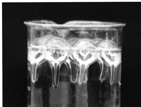
Fig. 1. A representative photograph of the TiO 2 -coated hollow pyrex glass beads floating in water.
